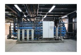
Fresh water can be produced from sea or brackish water, easily and in large quantities with a desalination plant. The sea water in high pressure will be separated in a reverse osmosis membrane. Energy is needed to run the pumps.
