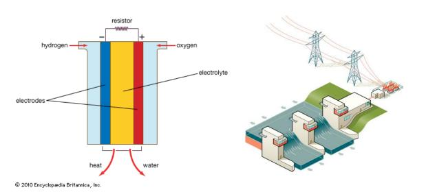
Water can be electrolyzed to produce Hydrogen for fuel cells. Fuel cells are "burning" hydrogen to produce again water and electricity. Can be used for vehicles or for any other kind of application
